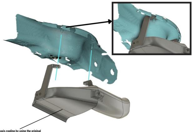
Assemble the rear axis cooling by using the original M6 bolts on the bottom of the whishbone.
