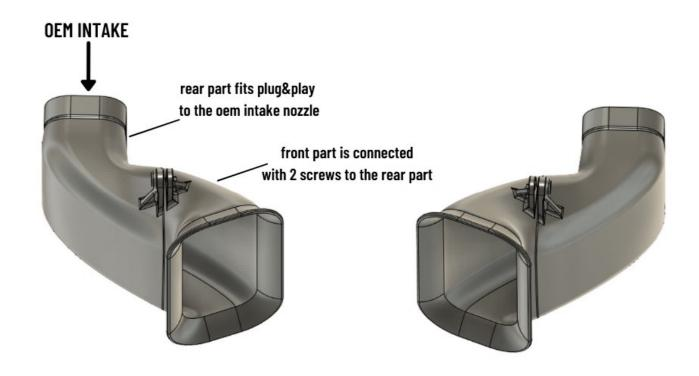
before connecting front and rear part, the cutting of the partition wall is required
