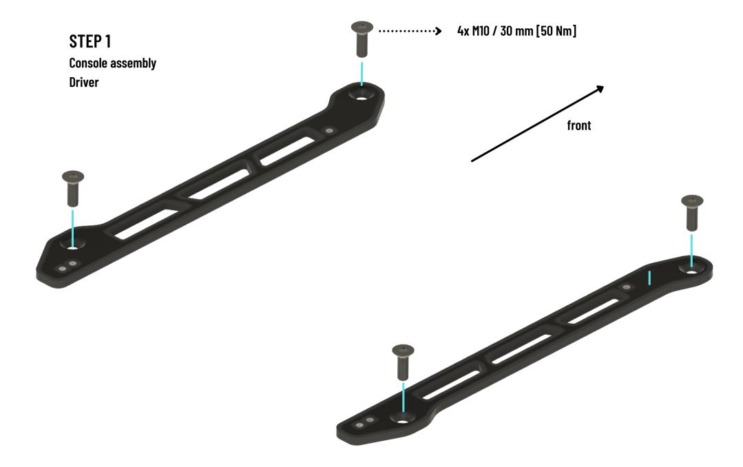
Please note! : If you're installing the co-driver seat mount, the parts need to be mounted mirrored.
