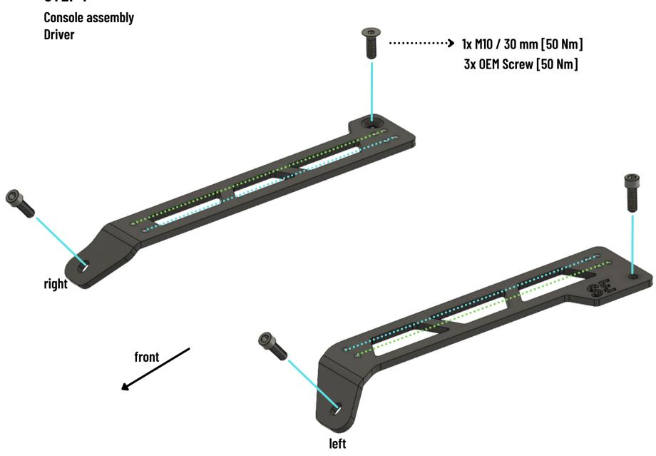
Use inner thread holes for the assembly of smaler seats like
