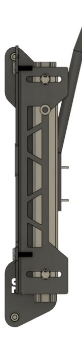
Adjust the seat position to the centre in front of the steering wheel. Tighten the screws and nuts as shown in Step 5 & 6.
