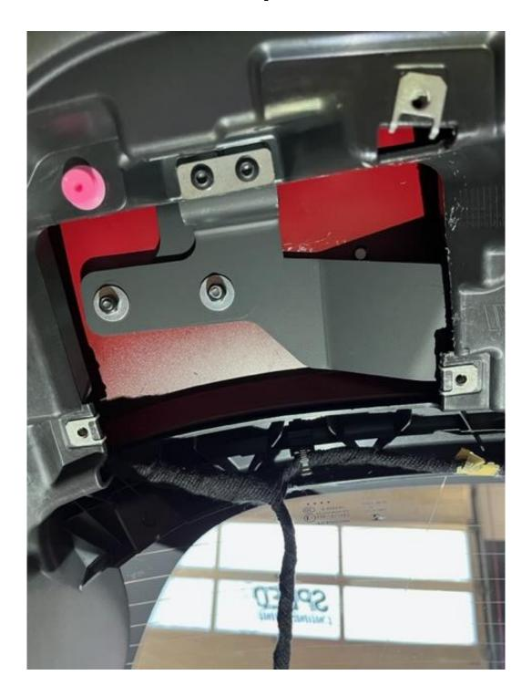
Fill the remaining holes (two per side) of the small reinforcement plate with the M6x25 lens head screws and the square washers.
