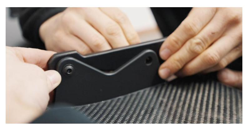
Install the aluminum adapters at the wing with two M6x10 lens flange screws and two M6 sleeve nuts per side. (May see step 16 for the correct mounting.)
