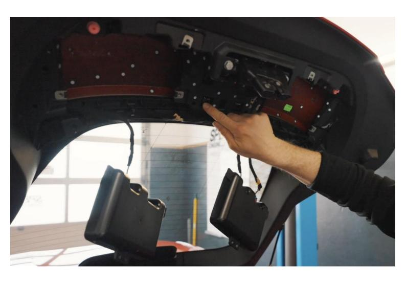
Drill the unused threads inside the trunk lid with a 8mm bit.
