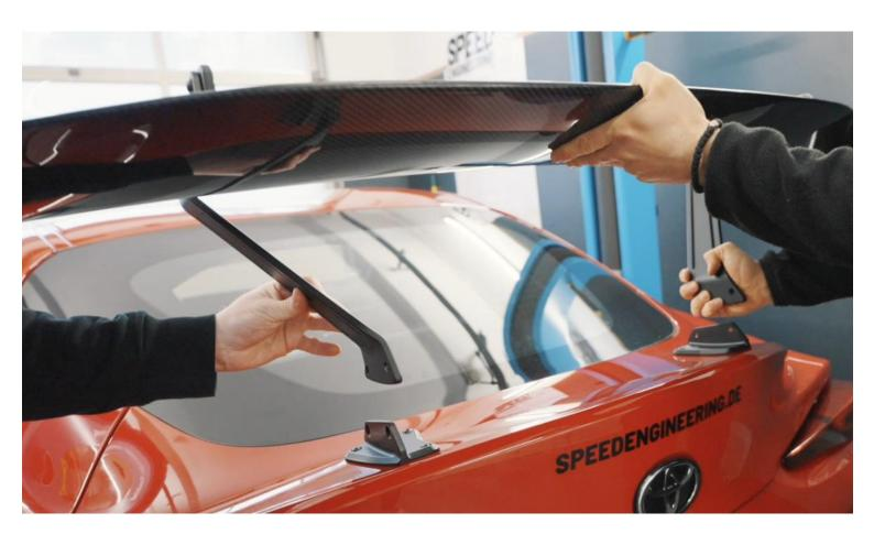
Finally mount the swan neck wing with the installed aluminum adapters at the aluminum stands on your trunk lid. Use the remaining M6 lens flange screws and the M6 sleeve nuts again.
