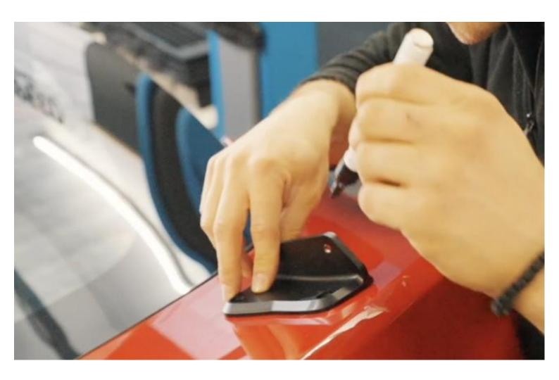
Close the trunk and align the CNC-milled aluminum stands at the trunk lid. The holes drilled in Step 6 should match the holes in the aluminum part. Mark the position of the third hole.
