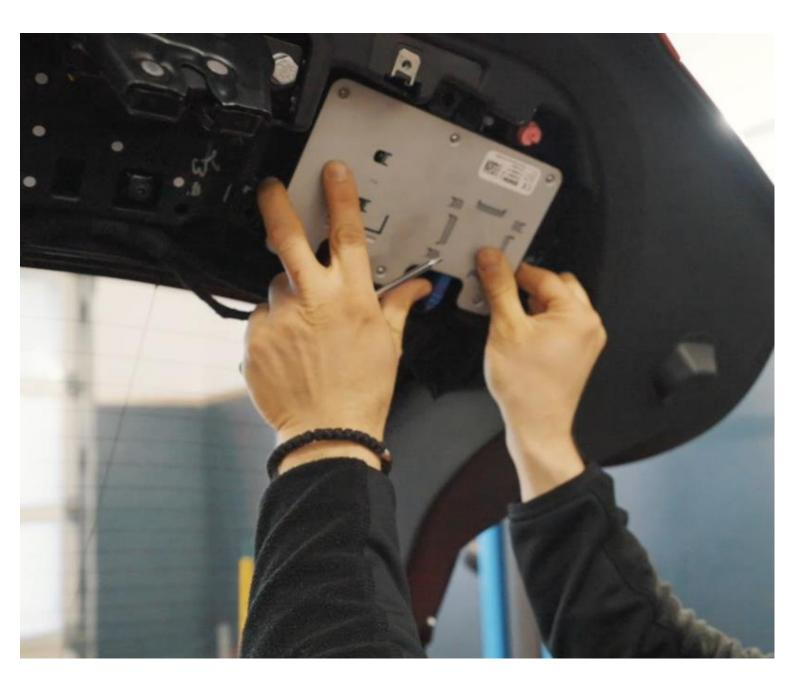
Mount the electronics again. Use only two screws per side instead of four at the given mounting points.
