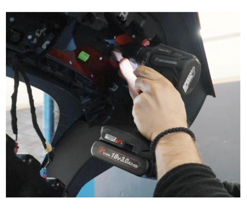
Drill the plastics trunk lid with a 7mm drill at the marked holes inside the reinforcement plate.
