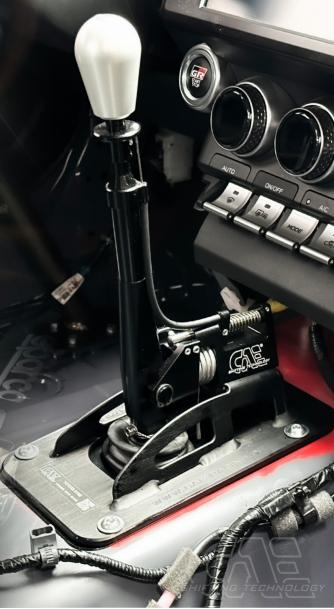
(i) The shifter is designed for vehicles with or without center console. For the installation of the center console, it must be processed according to these installation instructions until a corresponding clearance for the shifter is guaranteed.
