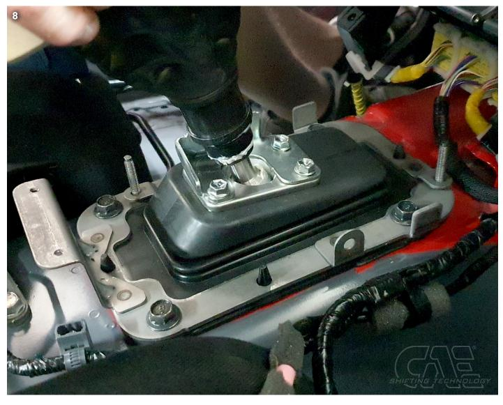
Unscrew the three screws of the bell lever bearing, as well as the 4 fastening screws of the center console support. Then remove the shift lever, rubber and frame. (Picture 8) ▶ Unscrew the rear bearing of the aluminum crossmember (2 x M8 screws), push up the two pin clips on the gearbox with a long screwdriver and pull the pins out to the side, then remove the shift lever bearing from the tunnel to the rear.
