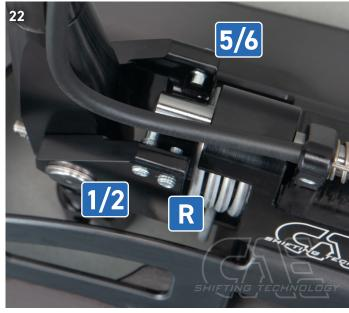
PLEASE NOTE: For gears 1/2 and 5/6, the grub screw must not touch the locking bolt when the gear is engaged!
