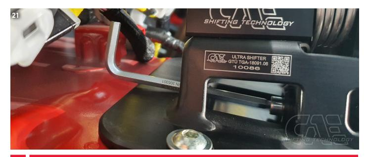
CHECK: When 3rd and 4th gear are engaged, the lateral clearance on the shift lever must be the same. If this is not the case, the spring stop must be readjusted. (0.5 mm is already a lot here).
