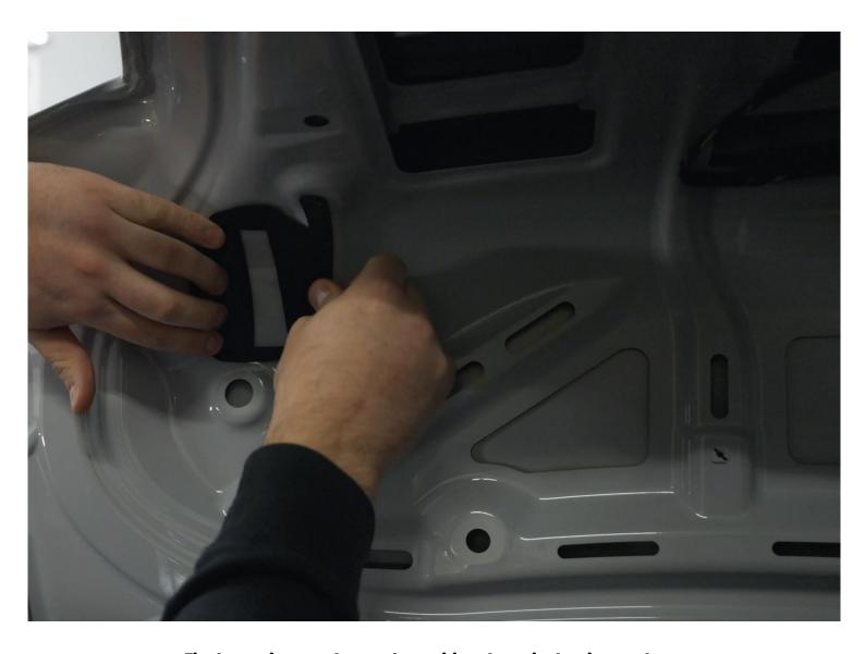
Fix the cutting template at the position shown in the picture above.
