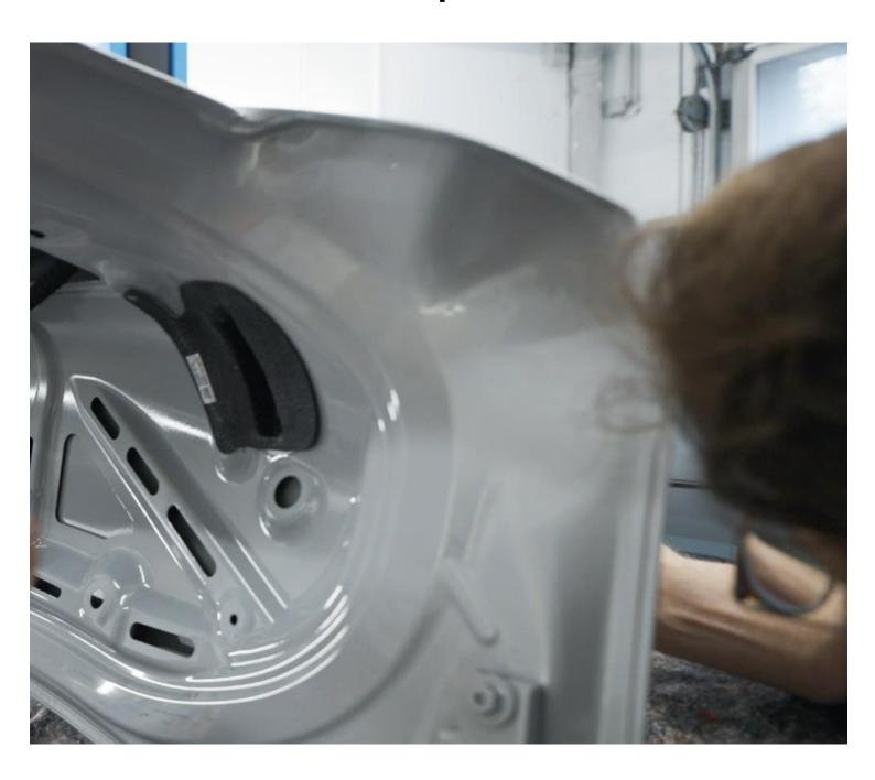
Press the reinforcement plate firmly against the trunk lid. It's good if the glue oozes out on the sides.
