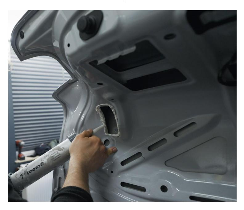
Apply adhesive for automotive parts all around the cutting edge. Please note: Apply to the cutting edges aswell, to protect the trunk link against corrosion!
