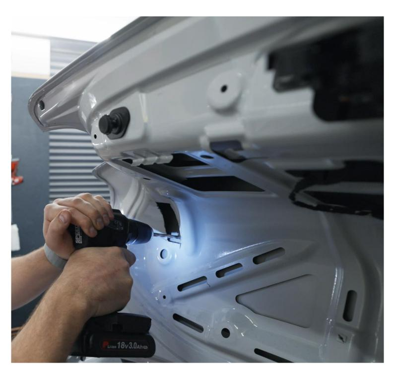
Drill the mounting holes: Both 6mm!
