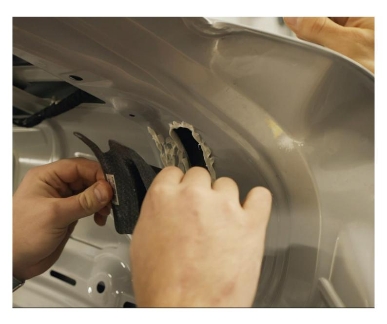
Fix the supplied reinforcement plates into the cutted holes.
