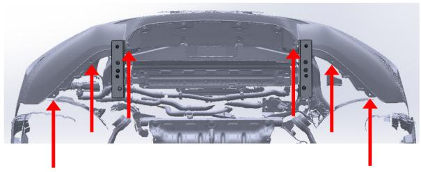
10. put the carbon lip on the bumper and use the OEM screws and M6 screws to attach it
