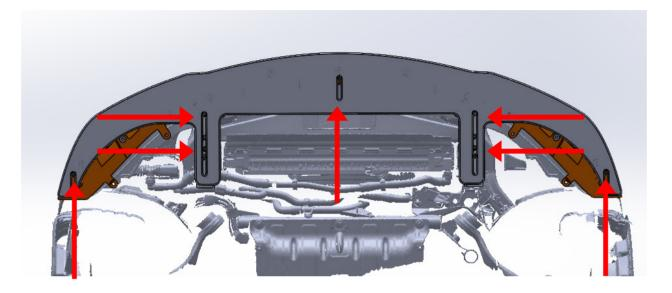
Due to tolerances, there may be a gap between the lip and the splitter board. To rectify this, the splitter board must be removed. After that remove the rear screws from the splitter holder and place the 1-3 washers supplied between the Blind rivet nut and splitter holder and tighten the screws again. Then assemble the splitter board. The gap is now removed
